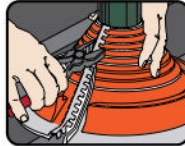
3. Squeeze joiner tightly with pliers to crimp
