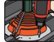
5. Fasten Retrofit to roof
