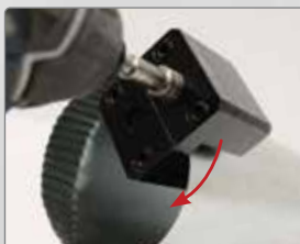
Exit crimping at slight angle
