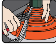
3. Squeeze joiner tightly with pliers to crimp
