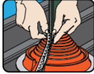
2. Wrap Retrofit around pipe, join the interlocking teeth
