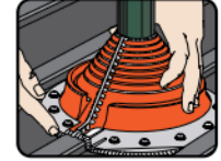
6. Apply additional sealant to mechanical locking joiner seam
